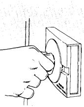
2. Turn cold control to OFF, and disconnect service cord from wall outlet.
